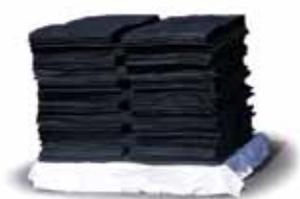
Masterbatch is an essential raw material which we formulate and compound in-house used in the manufacturing of our other tyre retreading materials. This is produced through a mixture of natural rubber and/or synthetic rubber, rubber processing oils, carbon black, chemicals and/or additives compounded with chemicals, such as sulphur, accelerators and/or other additives, to form the desired rubber compounds.
