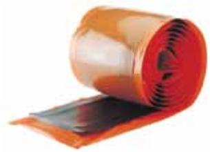
Camelbacks are unvulcanised rubber strips added to the surface of the buffed tyre casings. Camelbacks are mainly used in hot cure tyre retreading. These strips take the pattern of the mould during the process of vulcanisation.
